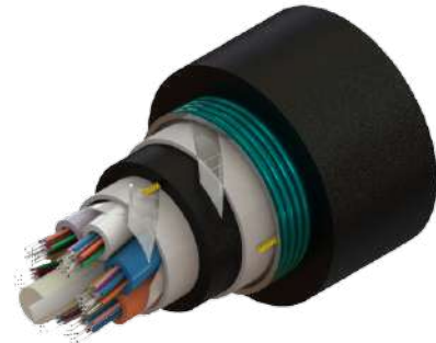
LOOSE TUBE SINGLE-ARMORED DOUBLE-JACKET CABLE DRY 72F G652.D FIBER FT
