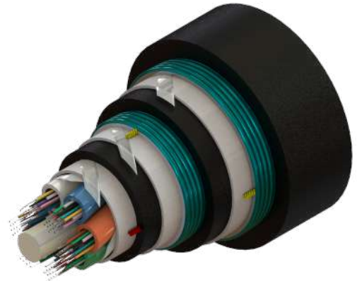
LOOSE TUBE DOUBLE-ARMORED TRIPLE-JACKET CABLE DRY 72F G652.D FIBER FT
